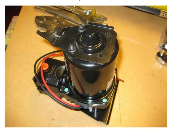
Now gently bend the bracket down, so the bend is close to the studs. Easy does it, you don't want to risk snapping those studs off.
