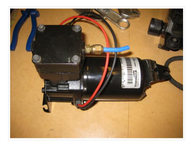
Remove the five 8mm bolts holding the bracket on the "big" end.
