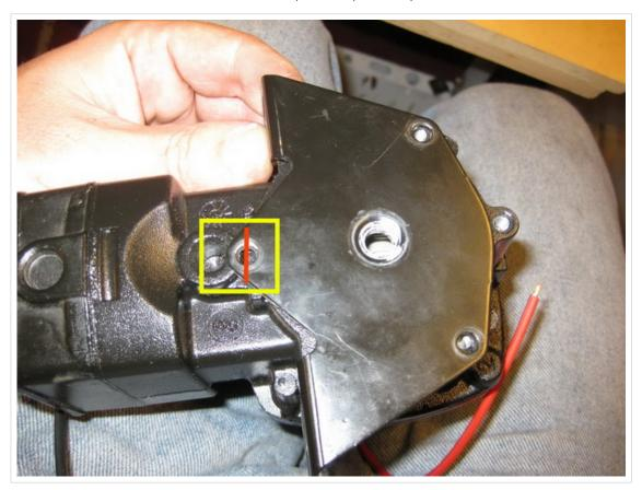
Using the new bracket as a template for where the two holes should be drilled in to the old bracket.
