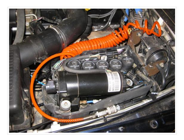
For safety, the EAS should be depressurised completely before doing any work on the system. Even though this operation should not affect the air already in the air-springs, you don't want to risk the car falling suddenly of high pressure air releasing when you don't expect it.
