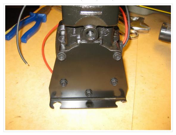
We are going to transplant the old bracket on to the new compressor, but the bolt holes don't line up, so we'll make a couple of new ones.
