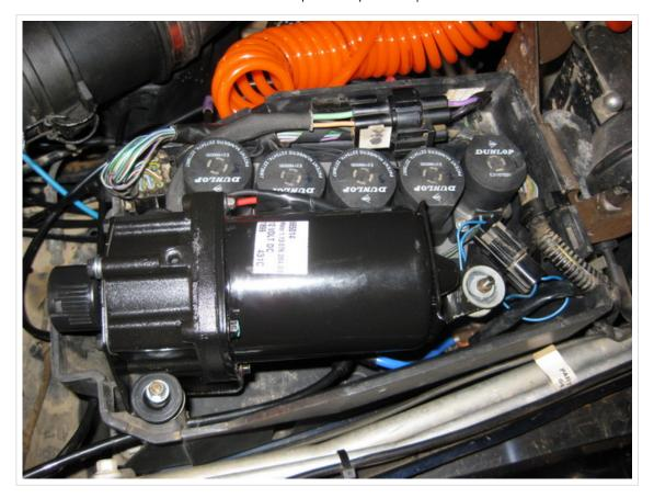
A stock EAS compressor is supposed to inflate the air tank from empty in about nine minutes. The Thomas compressor inflated my air tank from empty in four and a half minutes, or about half the time of a standard compressor!
