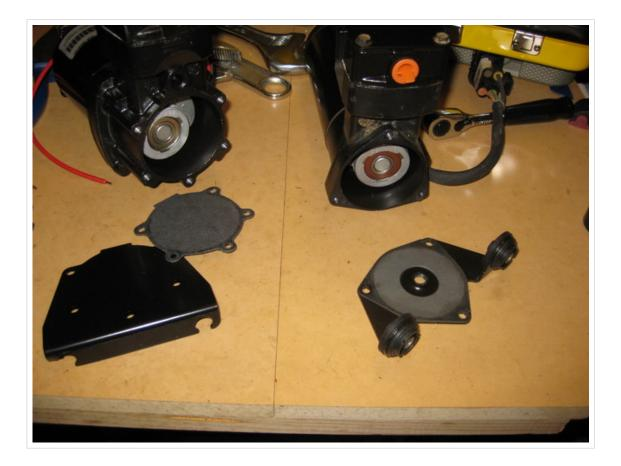
Trying the old bracket on for size. The mounting hole shown the yellow box below will foul on the body of the compressor, so we need to cut the bracket along the line shown in red.
