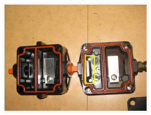
Apply a light smear of Vaseline to the gasket and o-ring before fitting the head.
