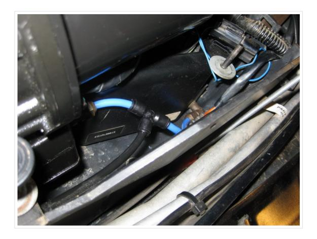
Back in place. Since the new compressor is wider than the original, the large washers would not fit on the mounts at the head end of the unit. I replaced them with 6mm washers.
