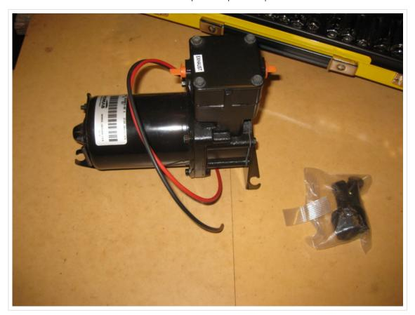
Remove the bracket at the "small" end using an 8mm socket.
