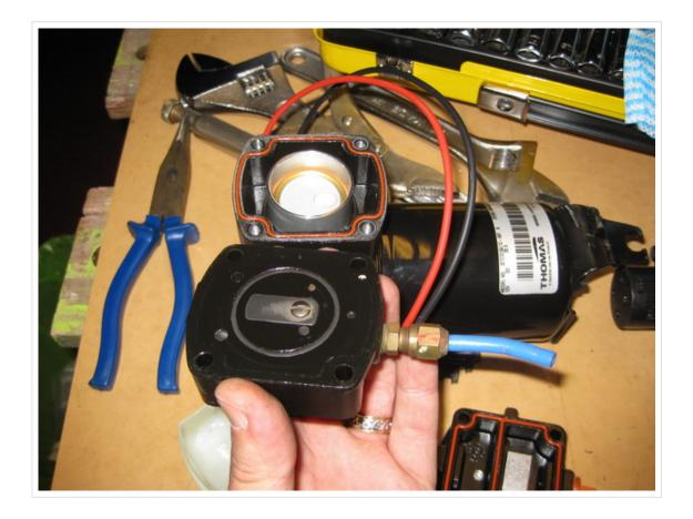
A bit more Vaseline to the orange gasket and put the head plate on.
